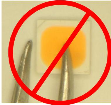
(2) In general, LEDs should only be handled from the side. By the way, this also applies to LEDs without a silicone sealant, since the surface can also become scratched.
