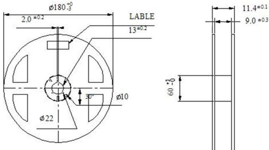
( Tolerance:  $\pm 0.2$ , Unit: mm )
